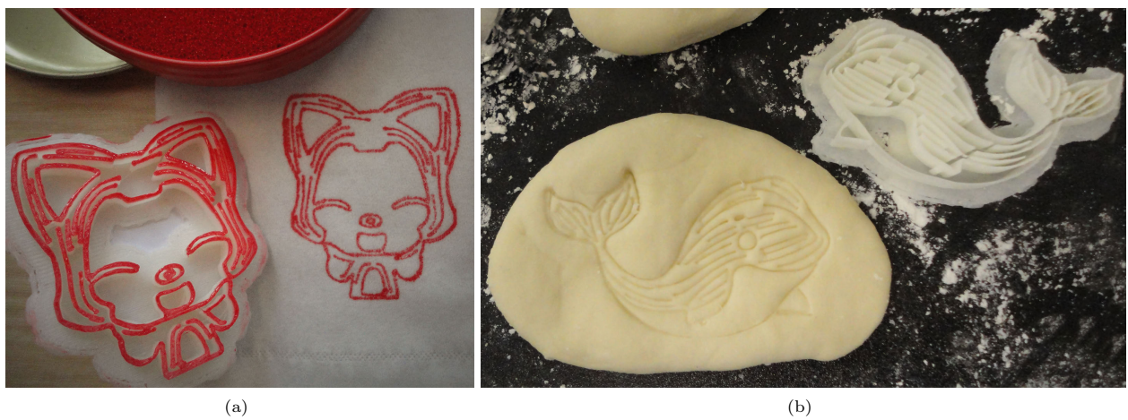
Figure 10: Photographs of 3D fabricated stamps. (a) A 3D printed stamp of 25 layers and a stamped napkin; (b) a 3D printed stamp of 40 layers and a stamp on a dough.
